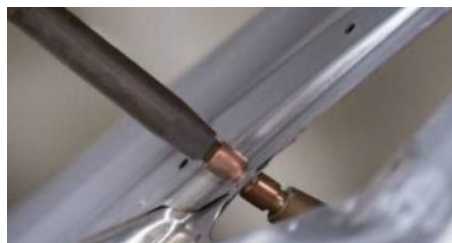
Aluminum Spot Welding
